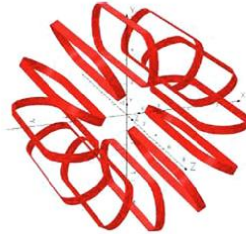
Figure 15. Racetrack Toroid System: This system utilizes superconductors in a toroidal design. The racetrack shape ensures a uniform distribution of the magnetic field, enhancing radiation protection performance while reducing mechanical stress on the superconductors. It is designed for effective shielding in space missions.[14]
